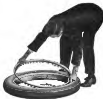
Fig. 5—Putting the outer rim in place
